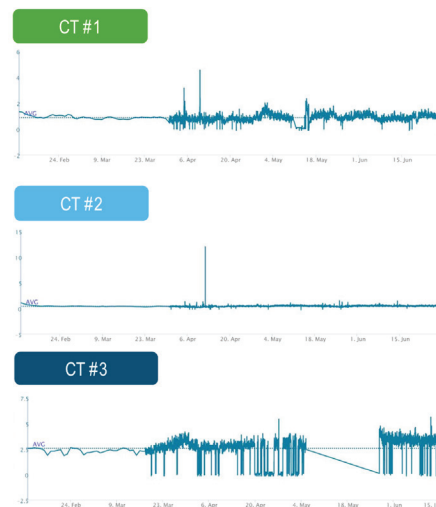
Figure 3. Average Steel Corrosion Rate. Corrosion rate for all cooling tower are maintained same as previous treatment program
